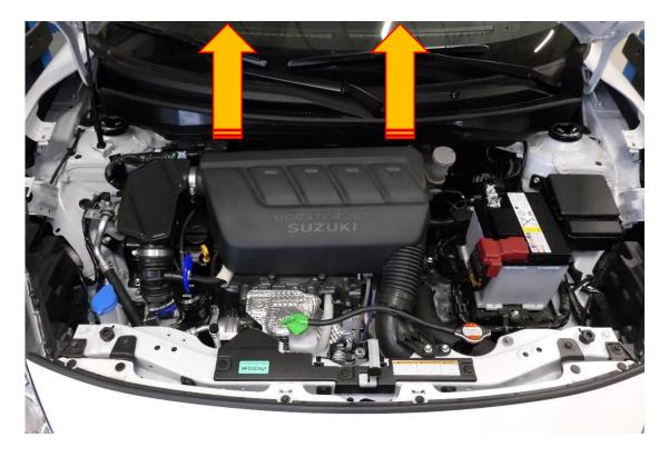
2. The air scoop/intake at the front of the engine bay is held down with four 10mm fasteners these need to be removed with a 10mm socket and drive. You can now remove the air scoop and hose (all three parts) from the engine bay.
