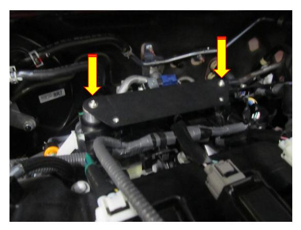
9. Take the hard pipe from the kit and mount the original MAF sensor into the MAF boss on the hard pipe ensuring the orientation is correct, there are two m4 fasteners with kit with the use of a 4mm Allen key tighten the sensor to the MAF boss.
