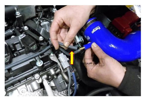
**16**. Remove the 10mm fastener shown in the picture ready to mount the Forge carbon air box.
