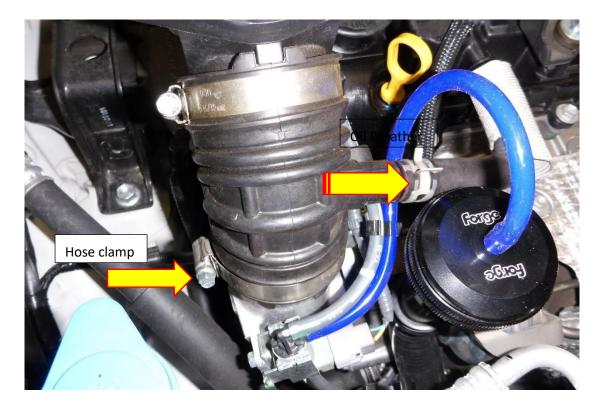
6. At this stage you can now remove the whole air box and pipe work as one, lift the back of the air box to release it from its rubber mounting points. Make sure all the vac hoses are unattached from the intake pipe and you will be able to remove the air box. To do this pull out the air box while twisting it 90 degrees to the left as shown in the picture.
