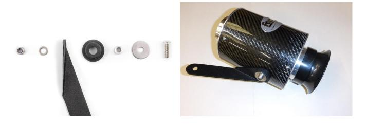
18. You can now fit the carbon air filter and bracket to the vehicle. (The recommended torque setting is between 2 and 2.4NM please do NOT exceed this or the alloy spinning on the filter will deform).
