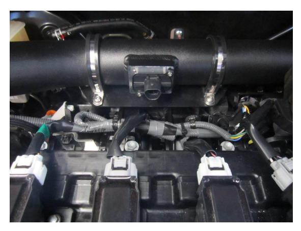
11. Now you can plug the MAF sensor loom back into place and cable tie down the excess loom with the injector loom as shown in the picture below.
