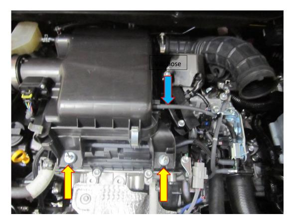
4. The MAF sensor will now need to be removed, first unplug the sensor then remove the two fasteners attaching it to the air box using a Pozi-drive screwdriver. Now carefully remove the sensor from the air box. Un clip the MAF wiring harness.
