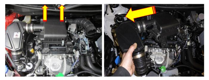
7. Now you can start to install FMINDK29, to start make up the hard pipe mounting bracket. Use the m6x6 fasteners and washers to attach both mounting pins using a 5mm Allen key as shown in the pictures below.
